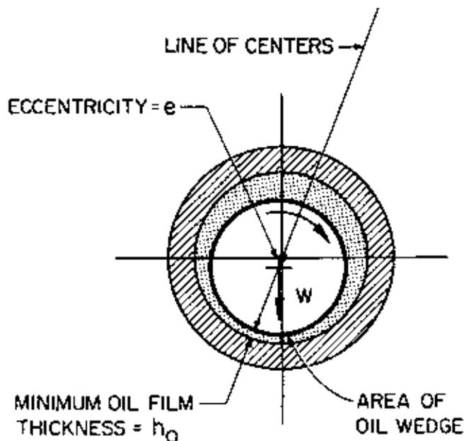
In the case of slow-speed engines, the oil pump, which is electrically driven, is turned on to prelubricate the bearings. This provides some lubrication. Nonetheless, bearings with liners and overlays are used to avoid seizure, which can result in costly damage.
