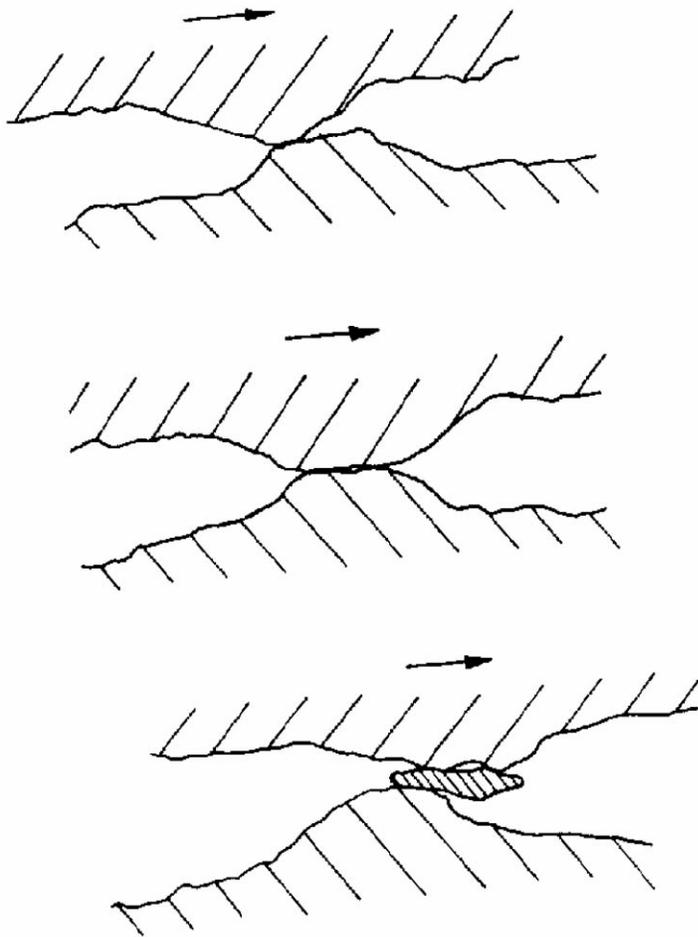
As a result of experiments carried out with various unlubricated materials—the vast majority being metallic—it is possible to write the laws of adhesive wear, commonly referred to as Archard's law, as follows [Archard, 1953]. For plastic contacts,
