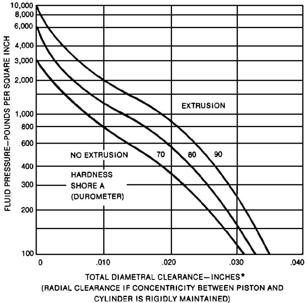
\*REDUCE THE CLEARANCE SHOWN BY 50% WHEN USING SILICONE OR FLUROSILICONE ELASTOMERS.
