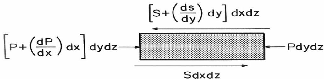
Substituting for  $(dS/dy)$  from Eq. (23.3) in Eq. (23.2), we obtain a second order partial differential equation in  $v$ . This is integrated to give the velocity profile as a function of  $y$ . This is then integrated to give  $Q$ , the total quantity of the lubricant flow per unit time. Applying certain boundary conditions, one can deduce the well-known Reynolds equation for the oil film pressure:
