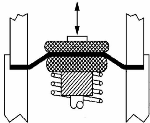
**Figure 24.24** Welded metal bellows.
