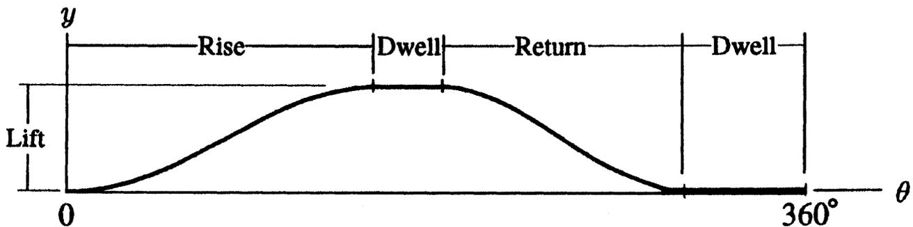
The cam profile is generated from the follower displacement diagram via graphical or analytical methods that use parabolic, simple harmonic, cycloidal, and/or polynomial profiles. For many applications, the follower's velocity, acceleration, and higher time derivatives are necessary for proper cam design.
