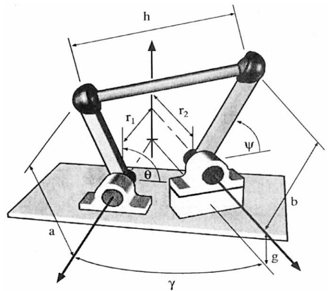
Another useful class of spatial mechanisms is produced by four hinges with concurrent axes that form a spherical quadrilateral known as a **spherical linkage**. These linkages provide a controlled reorientation movement of a body in space (Fig. 20.5).
