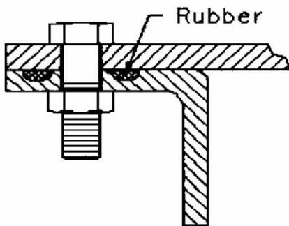
8. Formed in Place Elastomeric Gasket
