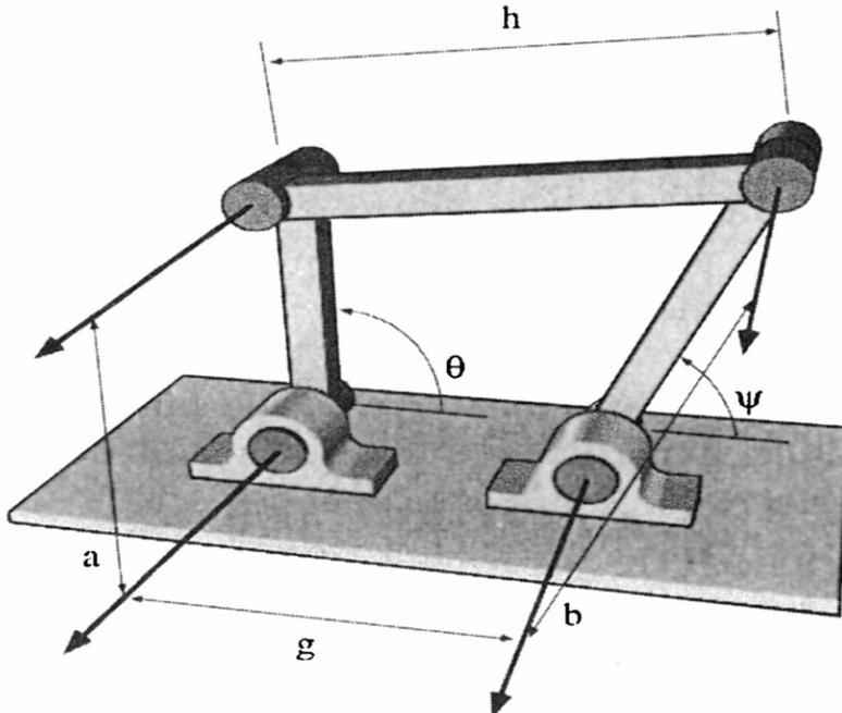
In each of these linkages a sliding joint, which constrains a link to a straight line rather than a circle, can replace a hinge to obtain a different movement. For example, a slider-crank linkage is a four-bar closed chain formed by three hinges and a sliding joint.
