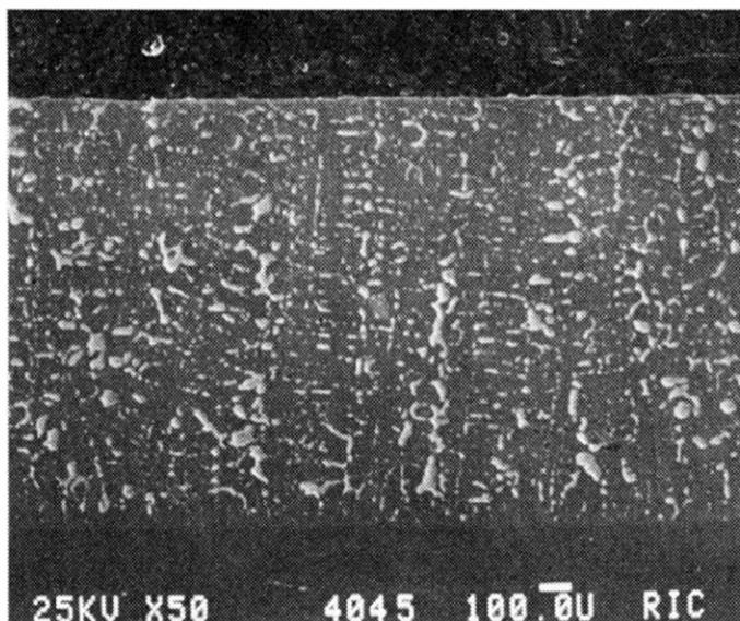
**Figure 23.4** SEM photomicrograph of a typical cross section of aluminum-tin material roll bonded to mild steel, manufactured by Glacier Vandervell Ltd. The nominal composition is 20% tin, 1% copper, and 79% aluminum. The light gray, irregular spots represent tin in the aluminum-copper matrix. Below the aluminum-tin layer is a layer of pure aluminum which functions as a bonding layer to the mild steel underneath. (Magnification 210×.)
