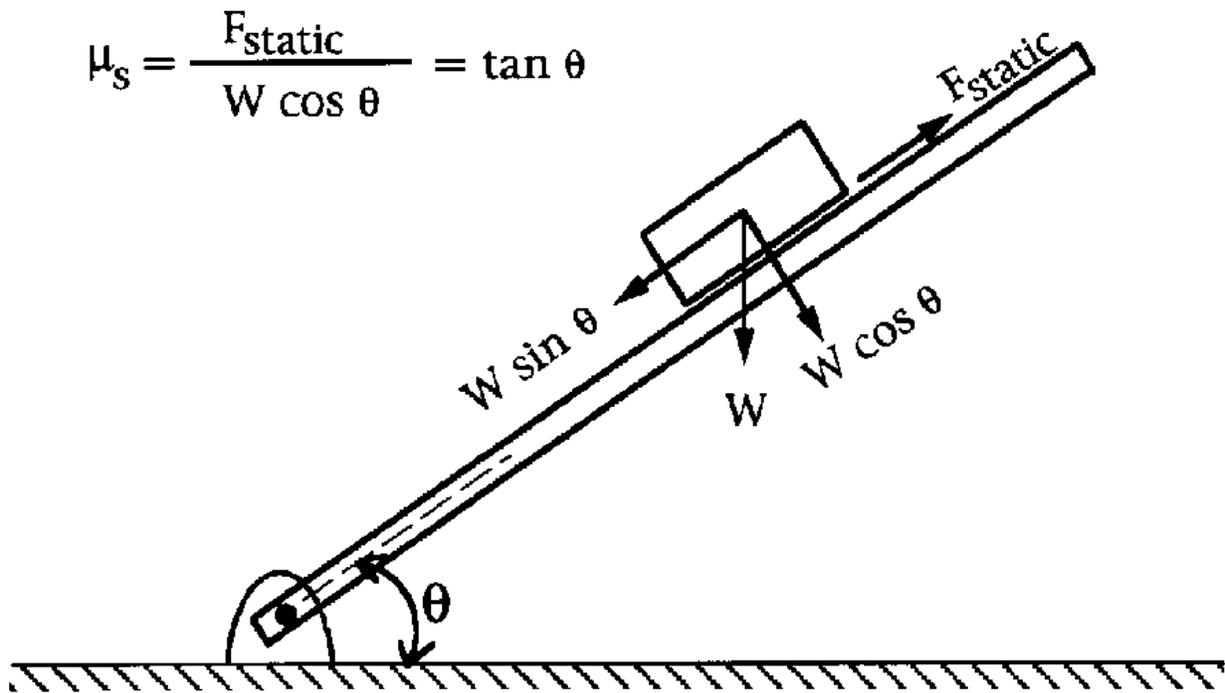
Typical values of coefficient of friction of various material pairs are presented in [Table 21.1](#) [Avallone and Baumeister, 1987]. It should be noted that values of coefficient of friction depend on the operating conditions—loads, speeds, and the environment—and the values reported in [Table 21.1](#) should therefore be used with caution.
