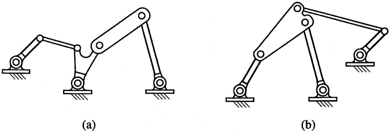
**Figure 20.3** Dimensions used to analyze a planar 4R linkage.
