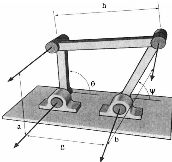
**Figure 20.5** A spherical 4R linkage.
