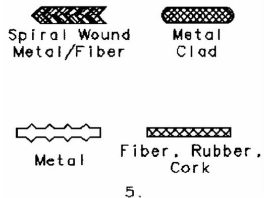
Gaskets can be made of relatively low-stiffness materials such as rubber or cork for applications at low pressures and where the surfaces are not very flat. For higher pressures and loads, one must utilize various composite materials and metal-encased materials as in Fig. 24.5.
