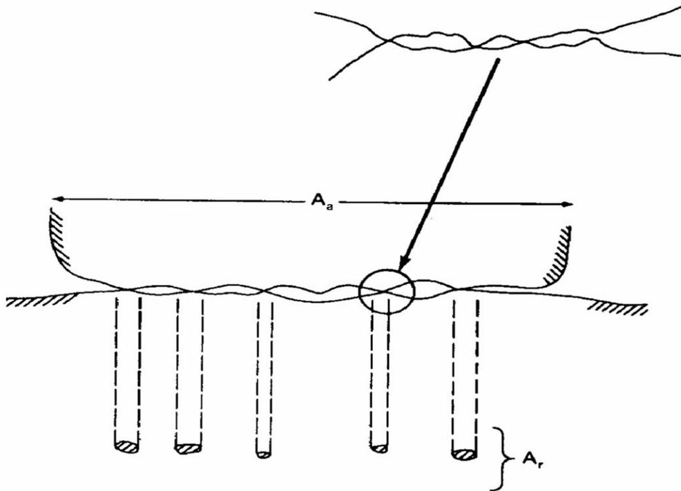
The contacts can be either elastic or plastic, depending primarily on the surface topography and the mechanical properties of the mating surfaces. The expressions for real area of contact for elastic ( $e$ ) and plastic ( $p$ ) contacts are as follows [Greenwood and Williamson, 1966; Bhushan, 1984, 1990]. For  $\psi < 0.6$ , elastic contacts,
