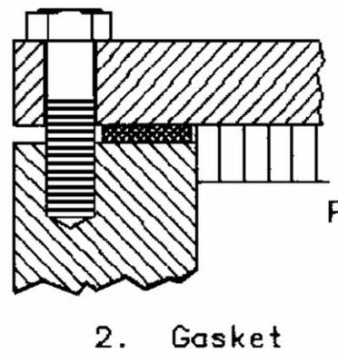
**Figure 24.3** Loaded gasket.
