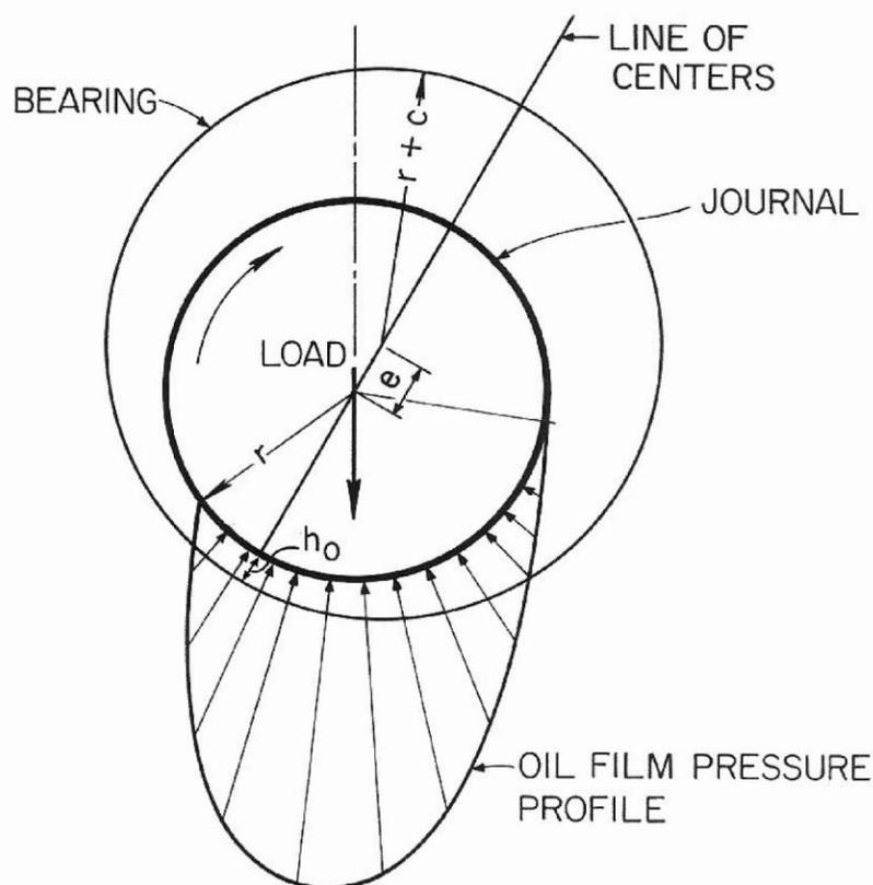
As a background to the theoretical considerations, the following assumptions are made. The flow of the lubricating oil around the journal at all speeds is assumed to be laminar. The length of the bearing  $L$  is assumed to be infinite, or the flow of the lubricant from the edges of the bearing is negligible. The lubricant is assumed to be incompressible.
